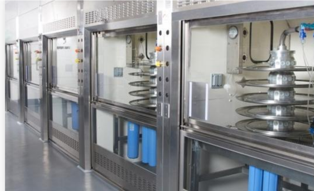
Flow-past inhalation exposure system with a syringe pump to clinical nebulizers (Sidestream) connected to high velocity airstreams
